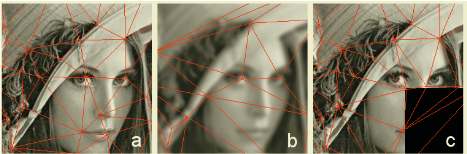
Fig. 1. Feature points and their Delaunay tessellation: (a) the original image, (b) the gaussian blurred image, and (c) the cropped image
