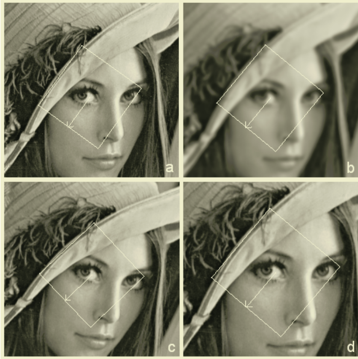
Fig. 5. The affine-invariant patch from the scale invariant feature transform: (a) the original image, (b) the blurred image, (c) the 10^\circ rotated image, and (d) the 1.2\times scaled image (the arrow represents the scale and orientation of the feature point)
